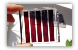
Figure 1: Mini-module (active surface area: 14 cm²) prepared with an organic dye synthesized in this work.
